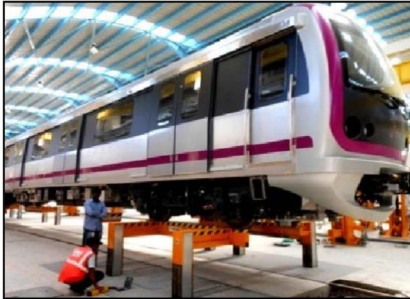
Synchronised Pit Jacks
